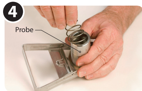
Install spring by placing the largest end of spring into the probe and wiggle in a clockwise direction while pressing down firmly.
