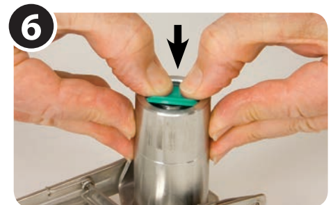
Place new dry break seal assembly on spring. Press the new dry break seal assembly firmly into the probe until the dry break seal locks into place.
