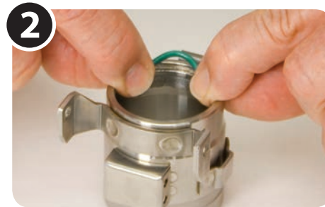
Install new O-ring seal into groove. Note: Lightly lubricate O-ring prior to installing with silicone grease or a lubricant that is compatible with the product. Take care not to spread the lubricant on other components.
