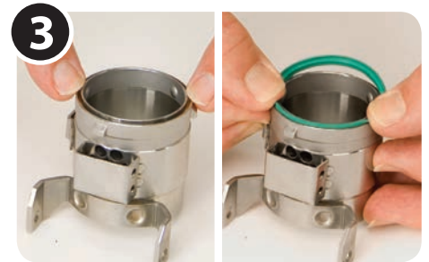
Turn coupler body upside down. Clean main seal groove. Install new main seal.
